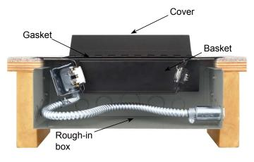
FMCA2000 assembly includes: Hinged Cover Integral Basket Cover Gasket Mounting Hardware Order Rough-in box and Moduline Insert Panels separately
