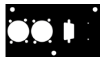
MPM 2ea Neutrik® D or 2eaSwitchCraft® D3F, 1ea VGA and 2ea pilot holes
